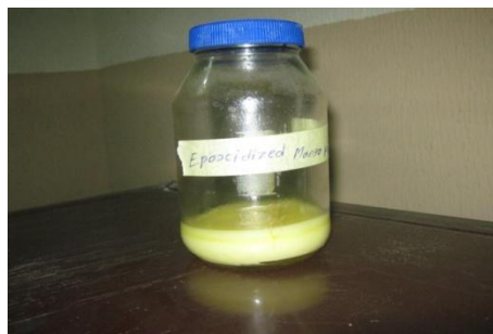
Plate 1: Epoxidized mango kernel oil (EMKO)
