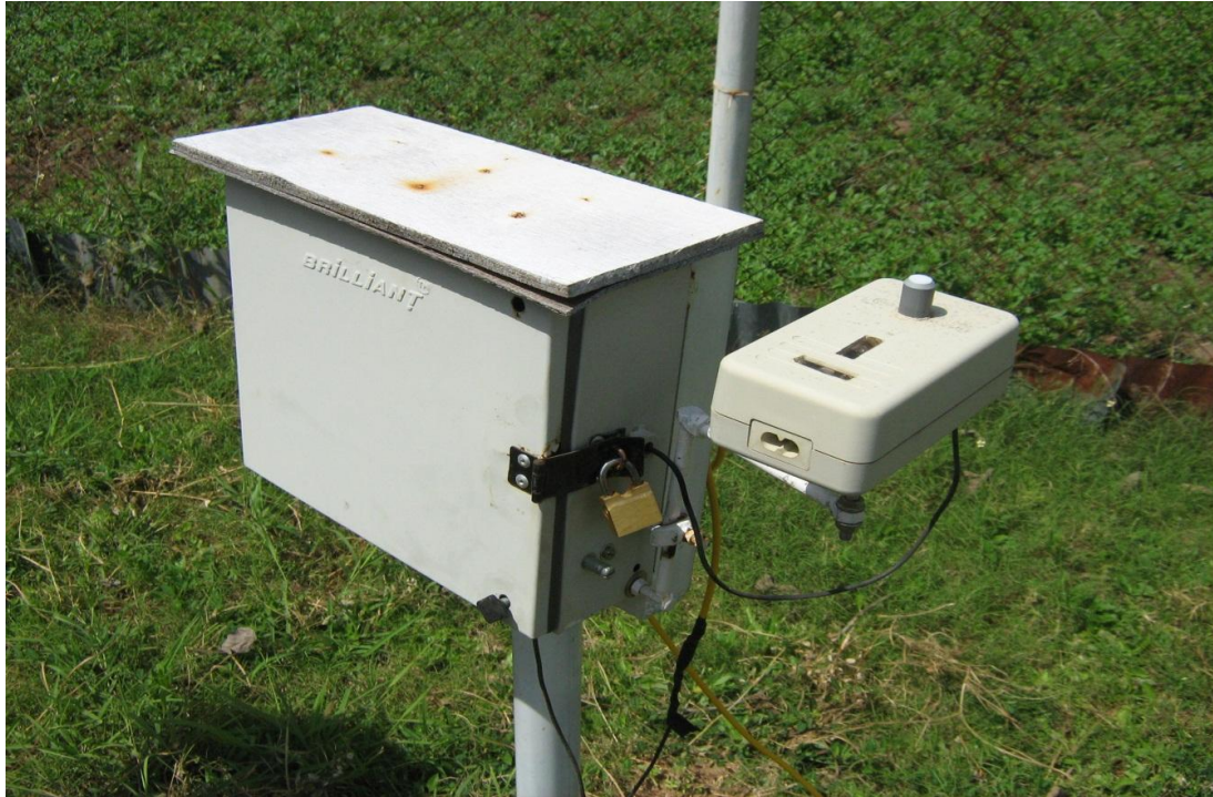
Figure 1. Picture of the constructed reliable model pyranometer (RMP001).
